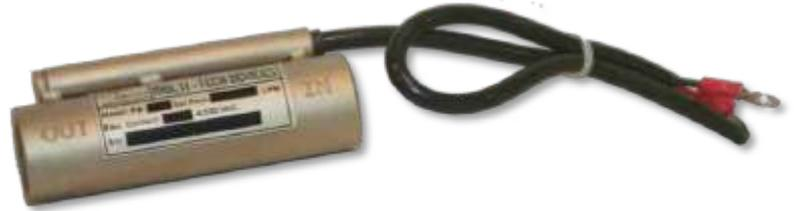
set point), after the enough flow passes through the flow switch the spring loaded plunger displaces in flow direction and actuates the Reed switch to give signal. Similarly when the flow decreases the plunger moves backwards and deactivates the reed switch. The FS-4D has generous internal clearances for reliability. The FS-4D is available standard with ½" BSPF connectons and in SS316 material.
