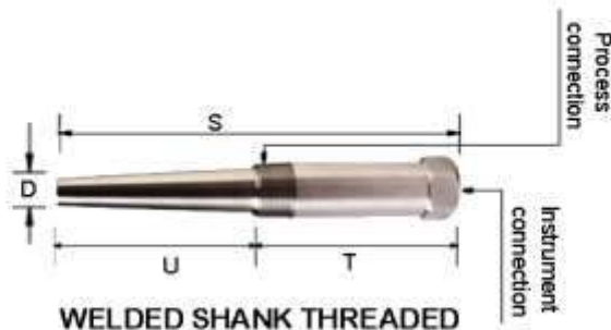
WELDED SHANK THREADED WITH LAG THERMOWELL
